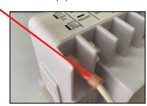
10. Use white/red harness from kit and connect end with smaller terminal to new timer (PWR).
