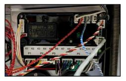
4. Remove old I/O module using phillips screwdriver.
