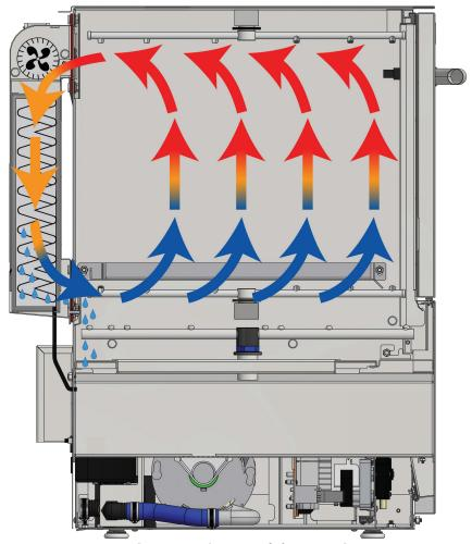
Cutaway side view of the HT-E-SEER
