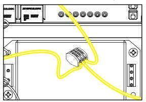
15. Connect loose end of WHT wire already attached to relay coil position 4 (on assembly from kit) to 3-position connector from kit.
