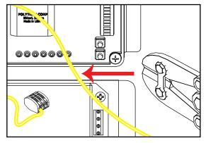
14. Connect both ends to 3-position connector from Step 11.
