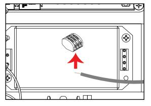
21. Connect loose end of GRY wire already attached to AC/L (on assembly from kit) to 3-position connector from Step 20.
