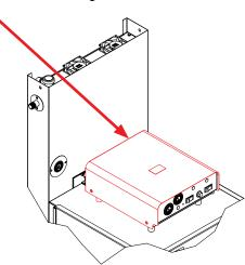
8. Remove control relay from studs using 5/16 nutdriver and keep hardware.
