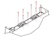
6. Connect BLK fan wires from new fans to connector with BLK wire from Step 2. Connect RED fan wires from new fans to connector with WHT wire from Step 2.
