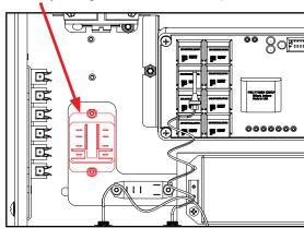
11. Connect loose end of YEL/WHT wire already attached to relay coil position 1 (on assembly from kit) to 3-position connector from kit.
