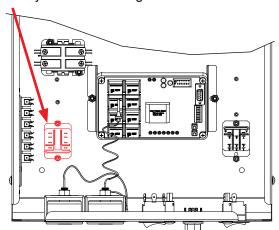
9. Install assembly from kit on studs from last step.
