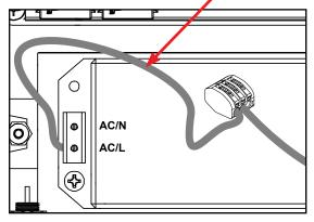
22. Attach RED wire with terminal already attached to AC/N and relay coil (on assembly from kit) to R2 coil.
