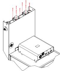
2. Disconnect four small BLK fan wires from connectors.
