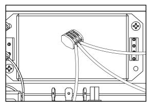
19. Follow wires from vent fan SJ cord. Locate where BLK wire terminates. Cut terminal off BLK wire, strip end, and attach to -Vo on power supply.
