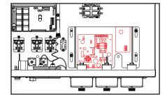
2. Slide POWER SWITCH on larger control board to OFF.
