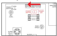
8. Turn DET. CON adjustment knob clockwise until detergent peri-pump starts operating.
