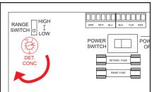
9. Turn DET. CON adjustment knob counter-clockwise until detergent peri-pump stops operating.
